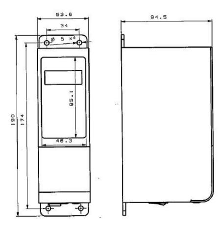
The controller is specially designed for controlling vibratory feeder in the automation systems. Combined with the latest electronic technology and elaborate design, the controller provides the following convenient and practical features:
